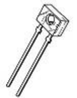
Cathode (lead on right looking from front)
